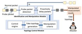
Fig. 2: The system architecture of ProTO.
